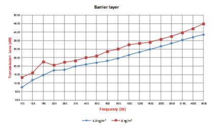
\*Results for 4.5kg m2 are tested to AS1191 Transmission loss report ATF-173 (revision 1)
